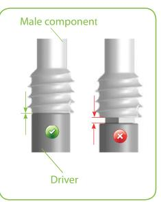
**5.2. LOADING OF THE FEMALE COMPONENT** To complete the screw assembly, simply slide the Female component onto the Male component up to the collar of the Male component.
