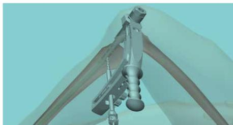
The one identified with the letter T permits the insertion of the corresponding drill bits supplied in the instrument box, which, when in place, will indicate the beginning of the tibial nail.
